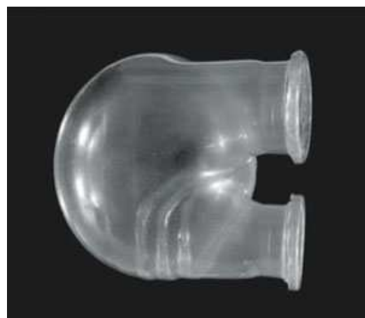
Figure 11 - Ventricular assist device chamber made of polyurethane: despite poor blood compatibility, it exhibits excellent abrasion and flexural properties
