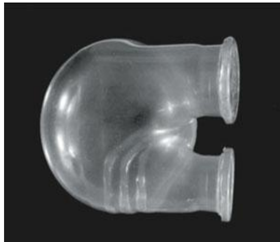
Figure 11 - Ventricular assist device chamber made of polyurethane: although it has poor blood compatibility, it exhibits excellent abrasion resistance and flexural properties
